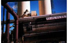
Double drum asphalt plant with 2 silos - one for hydrated lime & one for mineral filler
